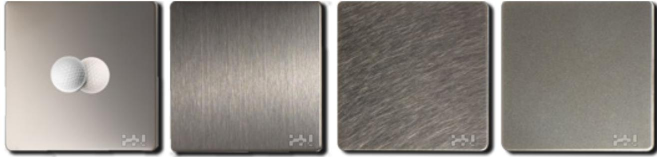
镜面灰钢 Mirror gray    拉丝灰钢 Hairline gray    乱纹灰钢 Vibration gray    喷砂灰钢 Sandblasted gray
