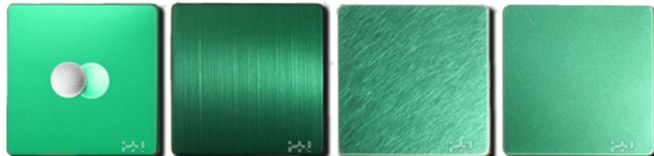
镜面翡翠绿 Mirror green    拉丝翡翠绿 Hairline green    乱纹翡翠绿 Vibration green    喷砂翡翠绿 Sandblasted green
